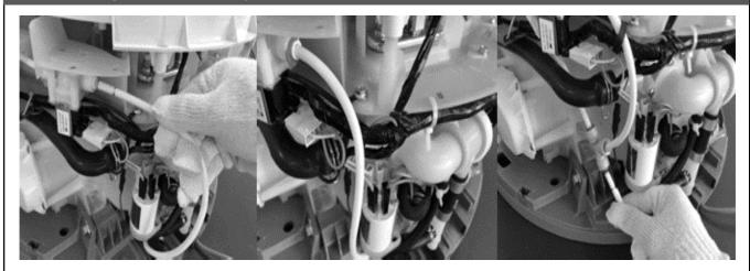
Insert the water inlet pipe into the water inlet valve coupling, minimum depth of 15 mm or more (black line on the hose) and install the retaining ring.
