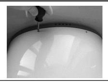
You have to remove the 2 screws from the top and bottom of the case to remove it.
