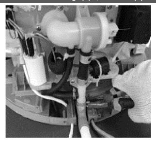
Attach the sewer hose to the drain connection and fix with the pipe clamp.
