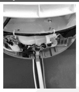
Place the water supply pipe and drain hose in the bushing of the housing. Make sure that none of the wires are kinked.
