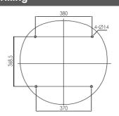
For the 4 suspensions of the machine for M10 or M12, drill screws in the attached mounting plate / support structure (drilling template enclosed). Alternatively, you can use the optional installation kit, in which the corresponding holes are already available.
