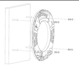
Fastening with 4x M10 screws and nuts, as well as washers and spring washers. Screws are guided through the wood reinforcement (see 2.a) and countered on the back with nut and washer. Alternatively, installation with original installation kit, available as an accessory, or by means of another supporting structure made of sturdy aluminium profiles (at least 40x40 mm) or comparable.
